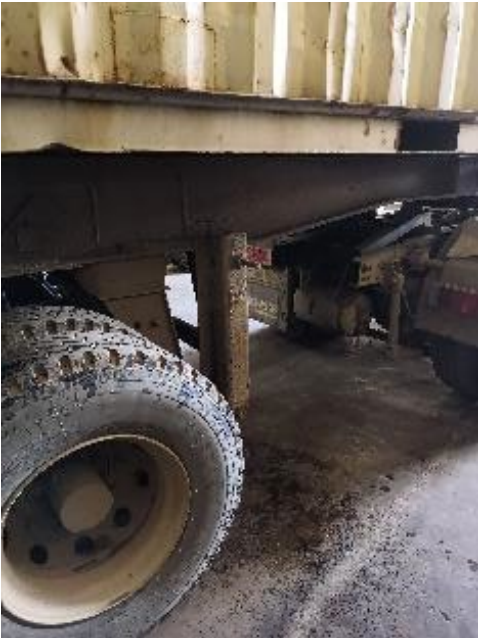
Oil leaking from container
